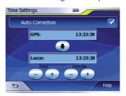
You can synchronise the Lucca's time with the GPS automatically or manually. You will also be able to change the synchronised time at a later date. You can also change the time if you selected automatic synchronisation.
